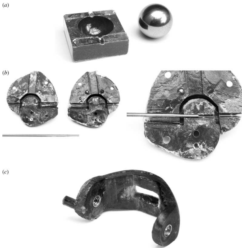
Figure 11. (a) Bearing ball used as a prototype of the yokes' spherical surface together with the negative of the half-sphere made in first phase of prototyping. (b) Vertical yoke mould components; note the metallic rod used to model the axle surfaces. (c) The vertical yoke ready for assembly.
