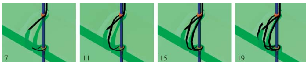
Figure 12. Sequence (selected frames) of laying down the carbon strand in the mould.
